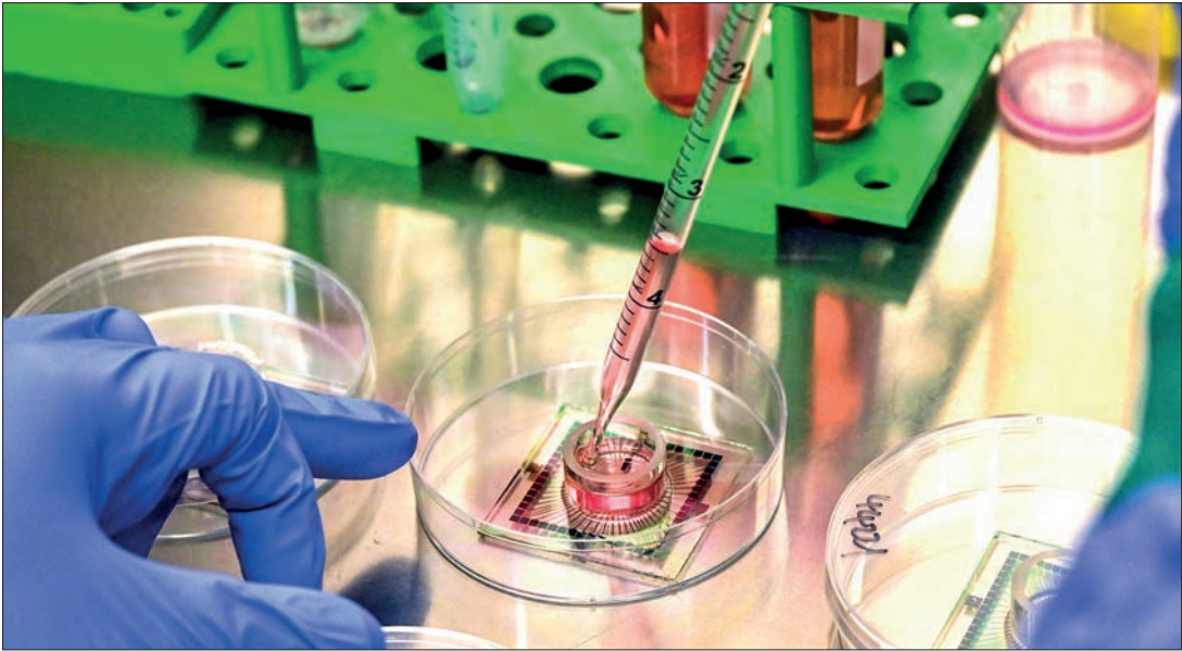
This photo taken on 5 May 2026, senior scientific specialist Kwaku Dad Abu Bonsrah pipettes nutrients onto neurons on Micro Electrode Array (MEA) chips at Cortical Labs' Physical Containment Level 2 (PC2) laboratory in Melbourne. PHOTO: WILLIAM WEST / AFP
